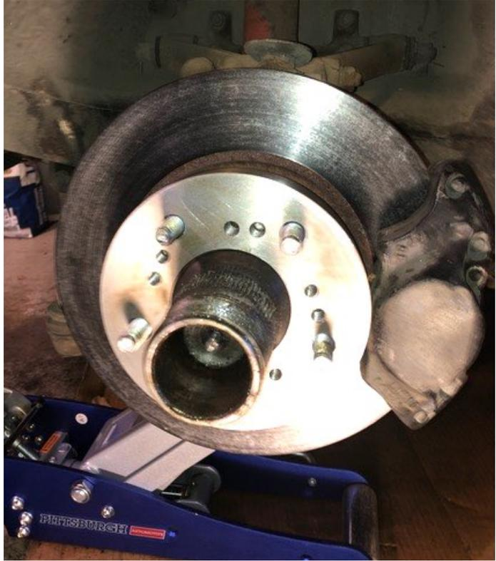
Duplicate set of holes for the brake rotor bolts on this prototype are due to communication error with the machine shop! → → → → →
